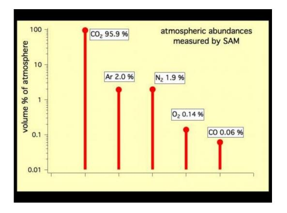
This graph shows the percentage abundance of five gases in the atmosphere of Mars, as measured by the Quadrupole Mass Spectrometer instrument of the Sample Analysis at Mars instrument suite on NASA's Mars rover in October 2012. Image Credit: NASA/JPL-Caltech, SAM/GSFC
