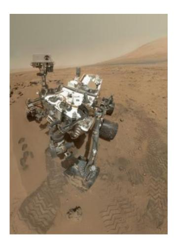
High-Resolution Self-Portrait by Curiosity Rover Arm Camera. On Sol 84 (Oct. 31, 2012), NASA's Curiosity rover used the Mars Hand Lens Imager (MAHLI) to capture this set of 55 high-resolution images, which were stitched together to create this full-color self-portrait. Credit: NASA/JPL-Caltech/MSSS
