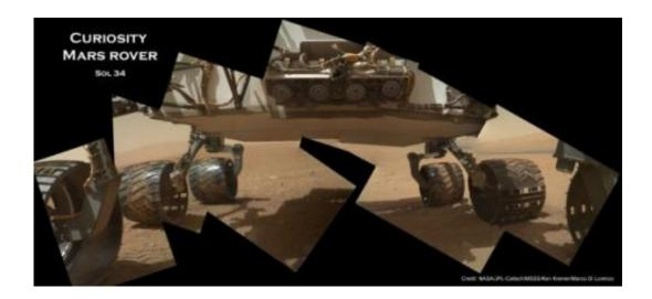
A mosaic of photos taken by the MAHLI camera on Curiosity's arm shows the underbelly of the rover and its six wheels, with Martian terrain stretching back to the horizon. Credit: NASA/JPL-Caltech/MSSS/Ken Kremer/Marco Di Lorenzo
