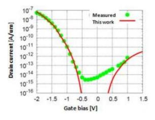
Comparison between measured values and results of a simulation of current–voltage characteristics of the tunnel FET Note: The difference in values near a gate voltage of 0 V is due to the leakage current through the gate dielectric layer observed in the measurement and is not specific to tunnel FETs. It can be suppressed by device design and therefore was ignored in the calculation.
