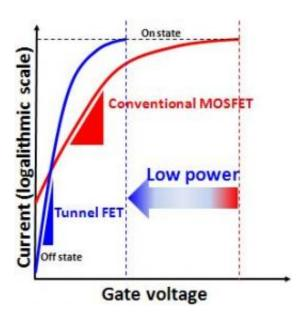
Steep switching characteristics of the tunnel FET.
