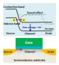
Structure and device principle of the tunnel FET. The dotted gray lines indicate the off state.
