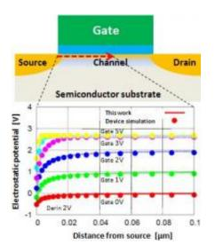
Comparison between the electrostatic potential distribution predicted by the compact model and numerical simulation results Electrostatic potential distributions in the direction of the arrow at the interface for different gate voltages (Vgs) are shown.
