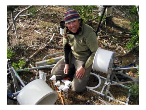
Mariah Carbone works on equipment used in the study of the microclimate where a Bishop pine forest is located on Santa Cruz Island. The large containers are automated soil respiration chambers, and the four small white pipes are soil carbon dioxide sensors. They allow the researchers to determine how much
