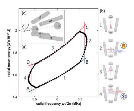
(a) Diagram of the Otto cycle for the radial mode of an ion. (b) Pictograms illustrate the four individual strokes of the Otto cycle. (c) Geometry of the tapered Paul trap used to trap the ion. Image credit: O. Abah, et al. ©2012 American Physical Society
