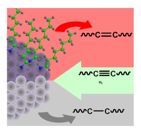
Alkyne hydrogenation on platinum nanoparticles with amine-coated (upper, red) and bare surfaces (lower, grey) produces alkene and alkane, respectively.
