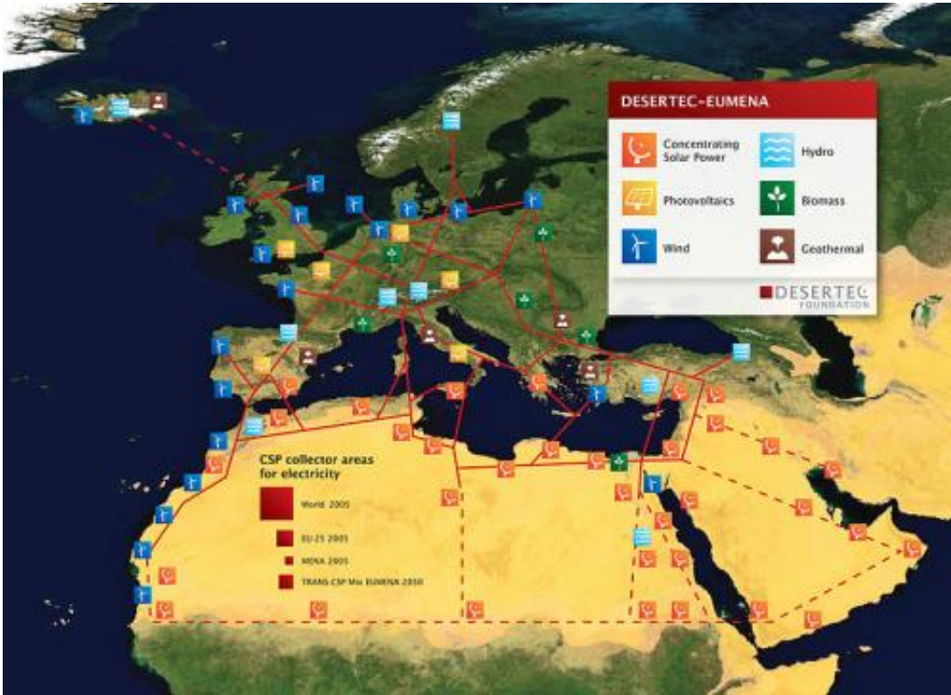
DESERTEC EU-MENA Map: Sketch of possible infrastructure for a sustainable supply of power to Europe, the Middle East and North Africa (EU-MENA) proposed by TREC
