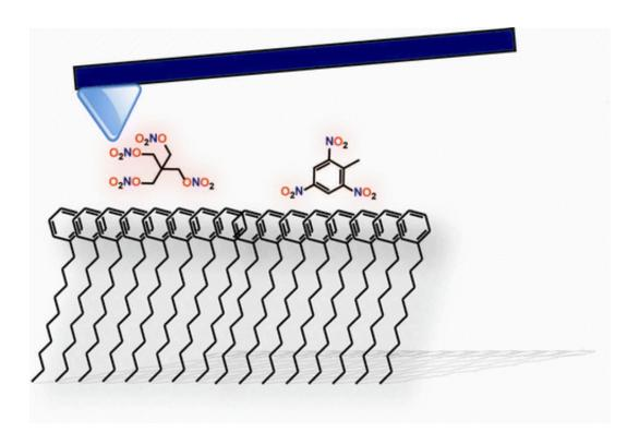
Using an <u>atomic force microscope</u> to measure the <u>adhesive forces</u> between explosive particles and different self-assembled monolayers, the scientists concluded that swab fabrics could be improved to collect smaller amounts of explosives by peppering them with hydroxyl, phenyl and amine <u>functional groups</u>. They believe that such additions could enhance the binding between the swab and irregularly shaped explosive particles.
