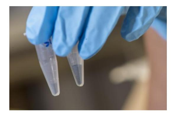
Rice University and Lockheed Martin have created a porous silicon powder that may lead to robust, powerful lithium-ion batteries. Fifty milligrams of the treated powder in the right vial has much more surface area than an identical weight of crushed silicon in the left vial. Credit: Jeff Fitlow/Rice University
