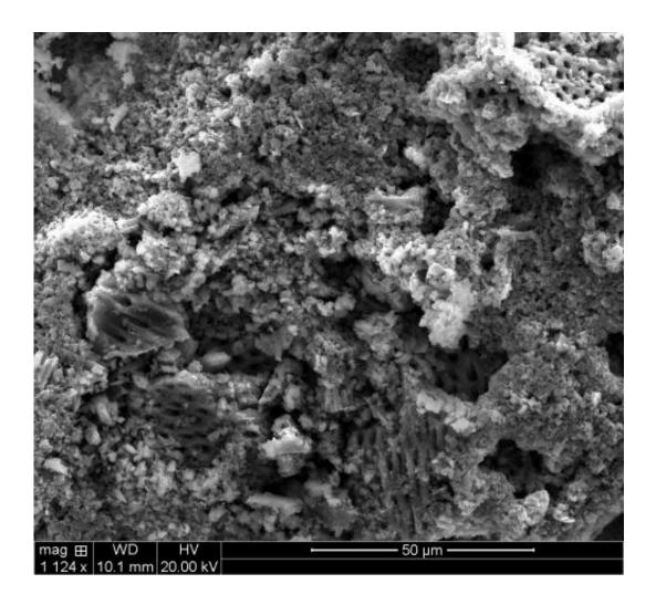
Porous silicon powder mixed with pyrolyzed polyacrylonitrile is the basis for a robust anode for lithium-ion batteries. Anodes developed with the powder at Rice University have achieved more than 600 charge-discharge cycles in the lab. Credit: Madhuri Thakur/Rice University
