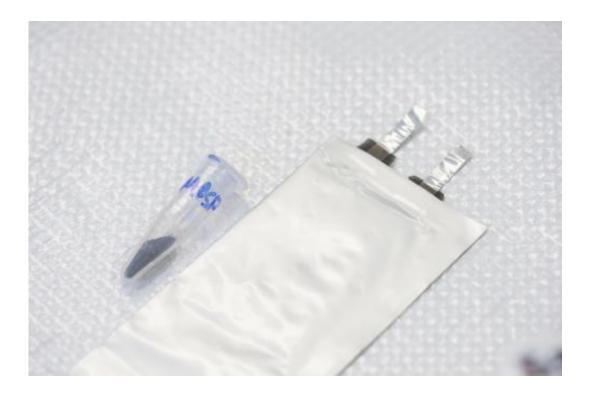
A half-cell battery that incorporates a porous silicon developed at Rice University has achieved more than 600 charge-discharge cycles in the lab. The work holds promise for next-generation batteries for electric vehicles. Credit: Jeff Fitlow/Rice University
