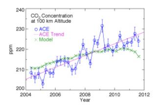
CO2 concentration at 100 km altitude (~62 mi) measured by ACE (blue circles) and predicted by a model of the chemistry and physics of the global upper atmosphere (green crosses). The purple line shows the linear trend of the ACE data. Credit: U.S. Naval Research Laboratory
