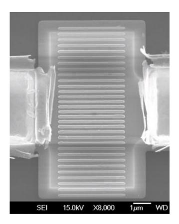
Crystalline silicon sits between two electrodes in a microscopic antenna-on-achip designed by researchers at Rice University. The chip, a spatial light modulator, couples with incident light and makes possible the manipulation of infrared light at very high speeds for signal processing and other optical applications. Credit: Xu Group/Rice University
