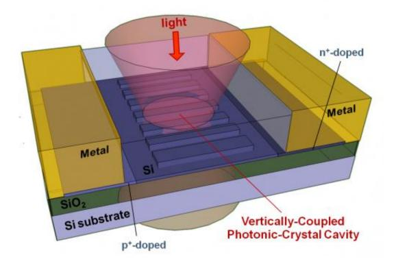
An illustration shows the design of Rice University researchers' antenna-on-achip for spatial light modulation. The chip is able to process incident infrared light for signal processing at very high speeds. Credit Xu Group/Rice University
