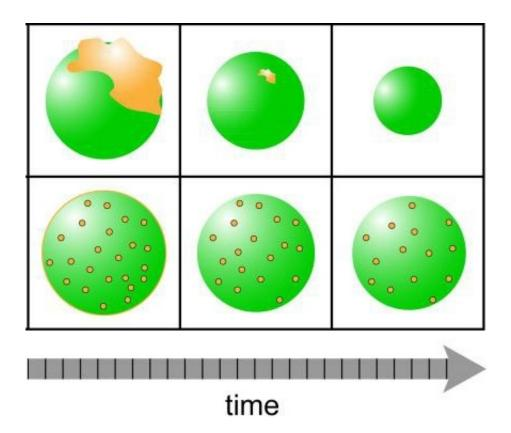
When airborne particles (green) form before pollutants known as PAHs (yellow) glob on, both the pollutants and particles dissipate quickly, as shown in the top row. But when the particles form in the presence of pollutants, which is what likely happens in nature, the long-lasting particles can take the pollutants for a long-distance ride (bottom). Credit: Zelenyuk/PNNL
