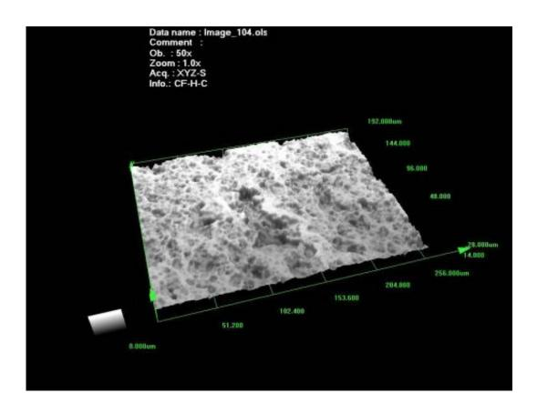
This is a close-up view of the highly porous, sprayable coating that Goddard technologists created to attract and then trap outgassed contaminants that harm spacecraft components. Credit: NASA
