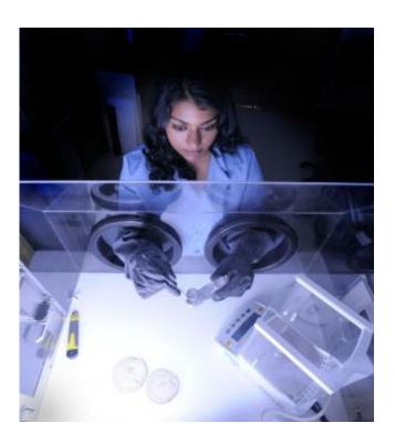
NASA Goddard technologist Nithin Abraham, a member of the team that has developed a low-cost, low-mass technique for protecting sensitive spacecraft components from outgassed contaminants, studies a paint sample in her laboratory. Credit: NASA/Pat Izzo
