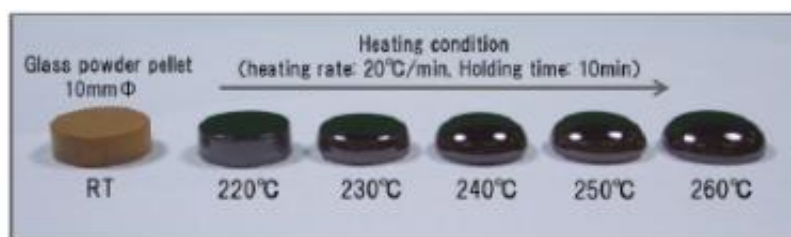
Softening flowability characteristics of the glass developed
