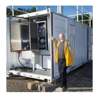
Brookhaven scientist Ernie Lewis and one of the mobile SeaTainer units now installed aboard the Horizon Spirit, a 272-meter cargo ship that will take atmospheric measurements during a yearlong cloud/climate study.
