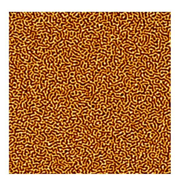
The picture of a 10µm by 10µm sample made with a magnetic force microscope shows the labyrinth-like structure of the magnetic domains. Credit: Bastian Pfau
