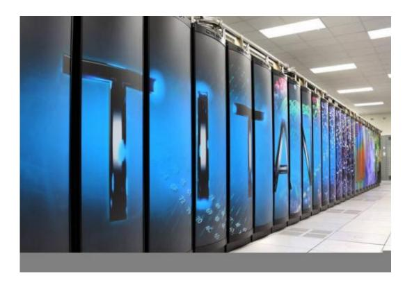
Titan is a supercomputer capable of churning through more than 20,000 trillion calculations each second -- or 20 petaflops -- by employing a family of processors called graphic processing units first created for computer gaming.
