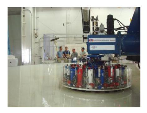
The first of seven mirrors for the Giant Magellan Telescope being polished at the
