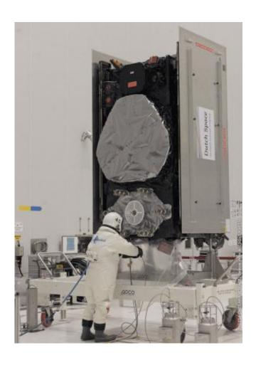
Galileo FM3 in the clean room at Europe's Spaceport, French Guiana. The fuelling process has begun ahead of the next Galileo launch in early October 2012. Credit: ESA/CNES/Arianespace/Optique Video du CSG
