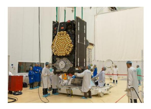
Galileo FM3 (Flight Model 3) undergoes a fitcheck for its dispenser at CSG, Kourou, French Guiana. FM3 will travel into orbit onboard Soyuz flight VS03, alongside Galileo FM4. Credit: ESA/CNES/Arianespace/Optique Video du CSG
