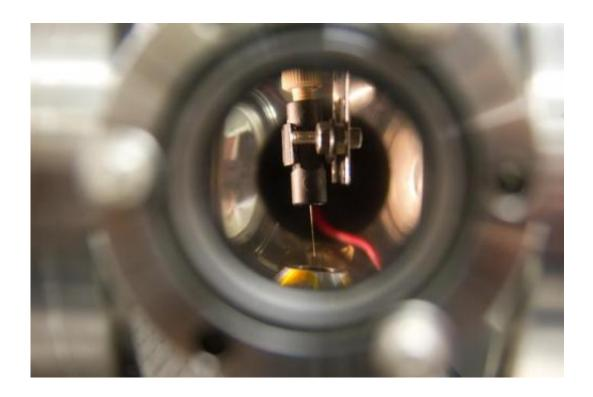
A liquid microjet, developed at SLAC, sends crystallized protein samples through a tiny tube, emerging in a thin stream in this vacuum-sealed chamber. Credit: Glenn Roberts Jr.
