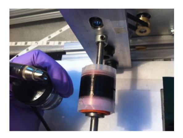
Researchers used a rotating spool to create ribbon-like composite material that have a high percentage of carbon nanotubes, for use in products from airplanes to bicycles. Credit: Yuntian Zhu, North Carolina State University
