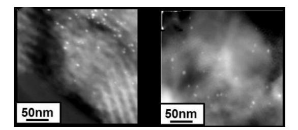
Heterogenized homogeneous nanocatalysts are sustainable as shown by these TEM images in which there is almost no difference in the cluster size of dendrimer-encapsulated gold nanoclusters (white dots) before (left) and after cyclopropanation reactions.
