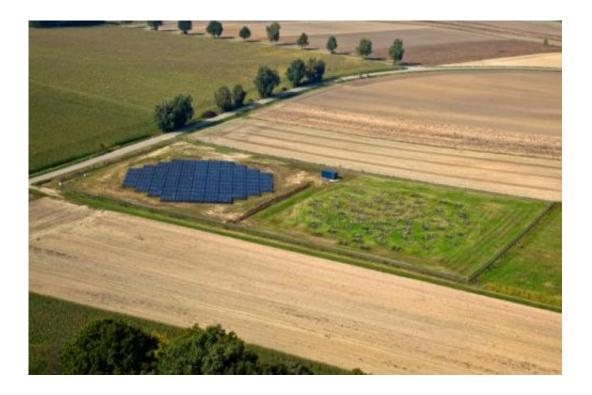
The LOFAR antenna array near Unterweilenbach is operated by the MPA. It is one of the 6 stations in Germany and 40 stations in the Netherlands that are combined to study the largely unexplored frequency range between 10 and 240 MHz. Image: Rainer Hassfurter/MPA
