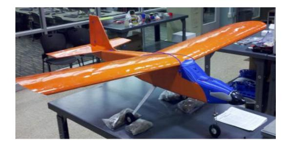
The unmanned aerial vehicle, "dressed" in U.Va.'s colors. The plane was built entirely from parts from a 3-D printer.
