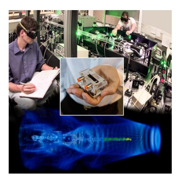
LOASIS has produced well-formed electron beams with energies up to a billion electron volts in laser plasma accelerators just 3.3 centimeters long. A typical
