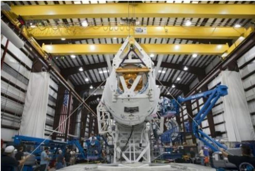
A photo released by NASA shows technicians as they attach the Dragon capsule to a Falcon 9 rocket at the SpaceX facility at Cape Canaveral Air Force Station in Florida on October 5. SpaceX aims for its next big launch into orbit Sunday—the first of 12 flights in its \$1.6 billion contract with NASA to bring supplies to and from the international space station.
