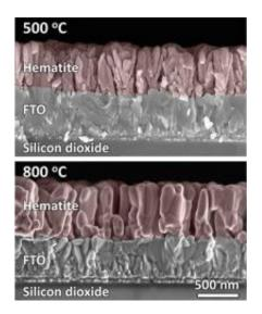
False-color scanning electron micrographs of cross-sectioned hematite films grown by sputter deposition and then annealed at two different temperatures. The physical structure and the tin dopant atom distributions in the hematite films differ depending on the annealing temperature. Hematite annealed at higher temperatures has better catalytic performance for splitting water.
