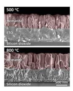
False-color scanning electron micrographs of cross-sectioned hematite films grown by sputter deposition and then annealed at two different temperatures. The physical structure and the tin dopant atom distributions in the hematite films differ depending on the annealing temperature. Hematite annealed at higher temperatures has better catalytic performance for splitting water.
