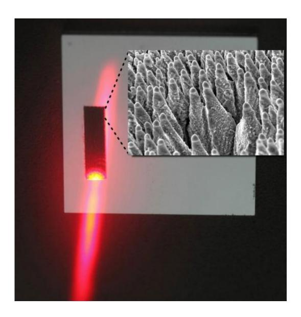
Black silicon is irradiated with a laser. Small image: Black silicon, magnified. Credit: Fraunhofer HHI
