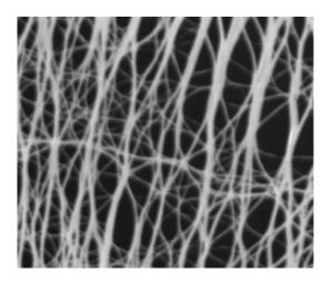
A thin film of pure carbon nanotubes produced at Rice University shows promise as a component of flexible, transparent touchscreens. Credit: Pasquali Lab/Rice University
