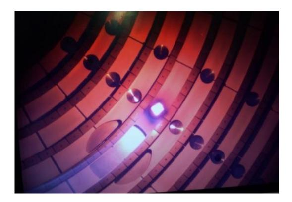
A heated electron emitting cathode (the bright spot at center) lights up the interior of a three-meter cast aluminum sphere used to contain plasmas, in an effort to create the kind of dynamo observed at the center of the Earth, sun and many other types of stars. Credit: Cary Forest laboratory
