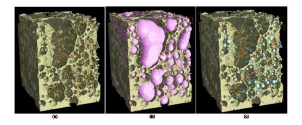
Example of skeletonization techniques used to measure bubble and pore throat sizes. a) The topology preserving skeleton with nodes shown in red at the intersections of the branches. b) The maximal inscribed spheres used to calculate the bubble volumes. c) The maximal inscribed spheres used to calculate the pore throat diameters. Wall thicknesses were also determined using maximal inscribed spheres. Credit: J. Fife/PSI; D. Baker/McGill University
