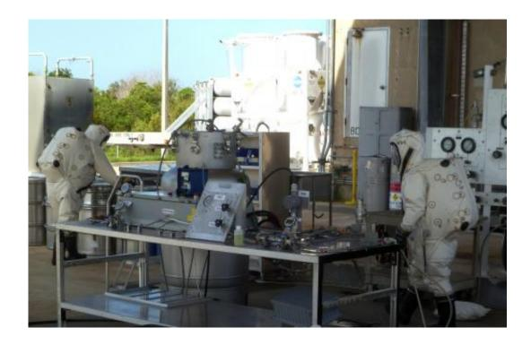
Wearing Self-Contained Atmospheric Protective Ensemble, or SCAPE, suits, technicians from Sierra Lobo conducted the first test of satellite refueling pump hardware to determine how it would perform with highly corrosive nitrogen tetroxide propellant such as that used by orbiting spacecraft. Credit: NASA
