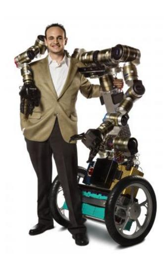
Georgia Tech assistant professor Mike Stilman poses with Golem Krang, a humanoid robot designed and built in Stilman slaboratory to study whole-body robotic planning and control. Stilman's research aims to give robots autonomous capabilities to perform rescues using tools found in the environment. Credit: Josh Meister
