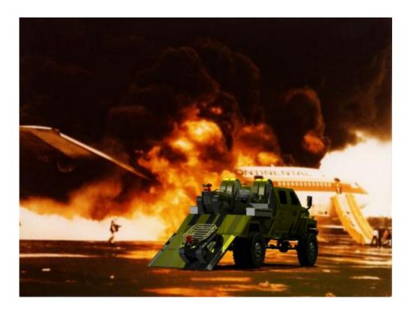
The Thermite is the centerpiece, a fire-fighting and emergency response robot propelled by caterpillar tracks which is remote-controlled from up to 1/4 mile away. The robot is hand-made from steel and aircraft-grade aluminum. The Thermite is small and compact enough to go through average door widths. Startup time to assume full robot functions is five seconds.
