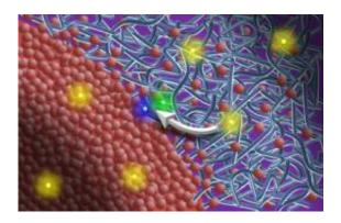
This is a molecular view at an interface between two regions in a solar cell. Red circles are buckyball fullerenes and are mixed with the blue spagetti-like polymer which work together to convert light into electricity. Credit: Image by Brian Collins for *Advanced Energy Materials*. Copyright Wiley & Sons.
