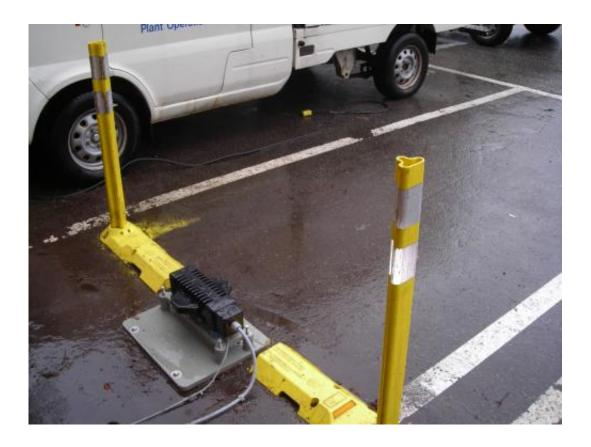
The new UBC wireless charging system works in all weather conditions. Credit: UBC
