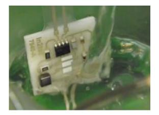
Recycling this printed circuit board is as easy as making a cup of tea - simply add hot water, and the bonding material dissolves away leaving you with 90% of your components to re-use as you wish.
