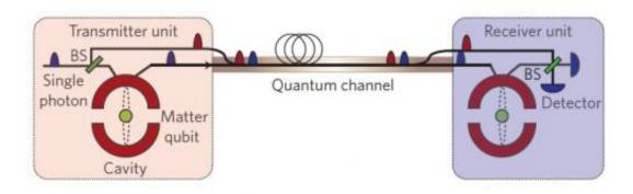
Illustration of the new quantum communication scheme, where information is directly transmitted from one node to another using a transmitter unit and a receiver unit. The scientists calculated that the new approach could potentially enable communication rates several orders of magnitude faster than other approaches. Credit: W. J. Munro, et al. ©2012 Macmillan Publishers Limited
