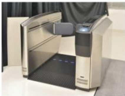
Prototype boarding gate with built-in explosives detection equipment
