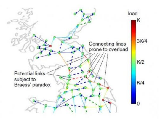
In this power grid model, the dashed lines represent potential new links at arbitrarily chosen locations. Two of these links (dashed red) are potentially subject to Braess's paradox and could destabilize grid operation. Braess's paradox can be caused by a nonlocal collective effect in which links in a nearby region are prone to overload. Credit: Witthaut and Timme. ©2012 IOP Publishing Ltd and Deutsche Physikalische Gesellschaft
