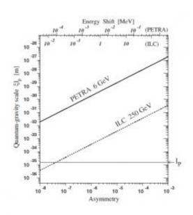
The PETRA-III accelerator at DESY and the proposed International Linear Collider (ILC) could test the energy-dependent bending of light by gravity at very small scales. Tests could measure two effects: refractivity, which produces energy shifts (upper scale) and birefringence, which produces a Compton edge asymmetry (lower scale). The Planck length is shown by an arrow. Image credit: Vahagn Gharibyan. ©2012 American Physical Society
