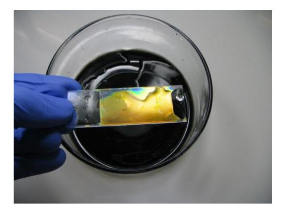
A photonic gel developed at Rice University and the Massachusetts Institute of Technology self-assembles from long polymer molecules. Polystyrene and poly(2-vinyl pyridine) are mixed in a solution that, when evaporated, allows the polymers to quickly form into nanosized layers. The layers can be tuned to reflect specific colors when exposed to particular chemicals. Credit: Joseph Walish/MIT
