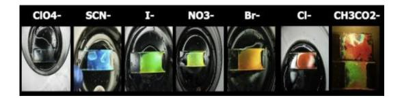
One photonic gel developed at Rice University was put through a series of color changes when repeatedly washed and exposed to new compounds. The gels show potential for inexpensive sensors and filters. Credit: Thomas Lab/Rice University
