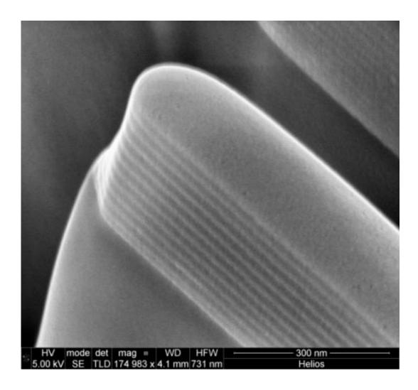
Alternating, nano-sized layers of hydrophilic and hydrophobic molecules selfassemble into a block copolymer called a photonic gel, developed at Rice University and the Massachusetts Institute of Technology. It changes color depending on the amount of water absorbed by the hydrophilic layers, which can be tuned by the solvent used. Credit: Thomas Lab/Rice University
