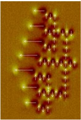
One nanoelectronics approach studied by the NRI MIND center is nanomagnet logic (NML)--logic circuits that work by magnetic coupling between neighboring nanoscale magnets. Here, SEM (l) and magnetic force microscope (r) images show an NML circuit that adds binary numbers. Credit: NIST
