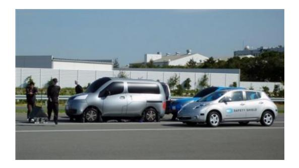
In this Friday, Oct. 12, 2012 photo, a Nissan car, right, tries to avoid a pedestrian dummy, second left, being pushed out by a Nissan worker, to a street behind the parked vehicles during a demonstration of "autonomous emergency steering" at the Japanese automaker's test ground in Yokosuka, south of Tokyo. The new safety technology is designed to avoid collisions through turns when braking would be too late. (AP Photo/Yuri Kageyama)
