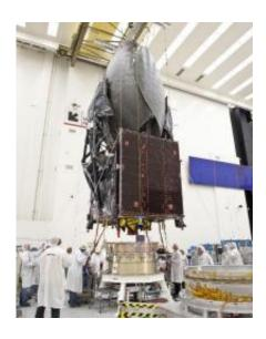
TDRS-K is in the Boeing satellite factory undergoing a fit check. Credit: Boeing Corp.
