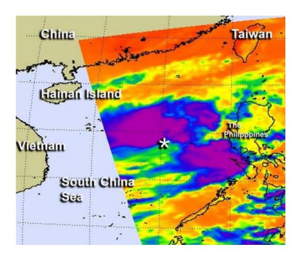
Infrared imagery from the AIRS instrument aboard NASA's Aqua satellite captured this image of Tropical Storm Gaemi on Oct. 2 at 0517 UTC. The purple areas indicate the most powerful thunderstorms with coldest cloud top temperatures. The asterisk (\*) indicates the center. Credit: NASA/JPL, Ed Olsen
