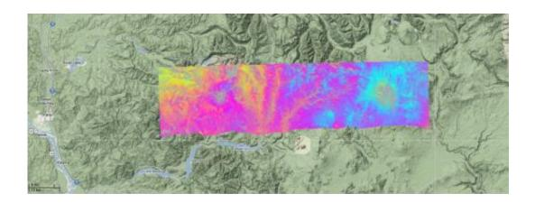
This UAVSAR interferogram shows active volcano Mount St. Helens (left) and dormant volcano Mount Adams, both in Washington state. The sensor collected data for this image during flights in July 2009 and August 2010 to compute the surface deformation that could indicate activity in the volcanoes' magma. No deformation was evident during this period. Credit: NASA
