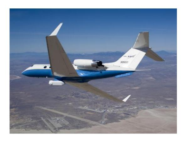
NASA's C-20A (G-III) banks over Edwards Air Force Base, Calif., carrying the UAVSAR underbelly pod, in preparation for studying U.S. and international volcanoes. Credit: NASA/Lori Losey
