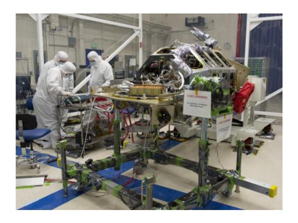
A team of engineers at NASA's Ames Research Center, Moffett Field, Calif., tests an electrical interface on the Lunar Atmosphere and Dust Environment Explorer (LADEE) spacecraft to ensure all of the cable pins are in the correct location and that it is safe to connect. Credit: NASA/Ames – Eric James
