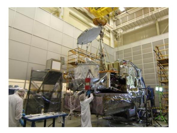
Engineers check on the GPM spacecraft after successful completion of its first comprehensive performance test. The silver disc and drum (center) is the GPM Microwave Imager, and the large block on the base is the Dual-frequency Precipitation Radar. The tall golden antenna is the High Gain Antenna for communications. Credit: NASA
