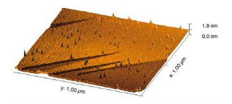
Following bombardment with highly charged ions, nano-hillocks have formed in an area of localized melting. This is an atomic force microscope image. Credit: HZDR
